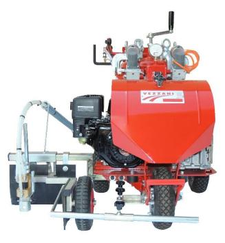
*Engine* : petrol , 6.5 hp with recoil starter and clutch to facilitate starting.
