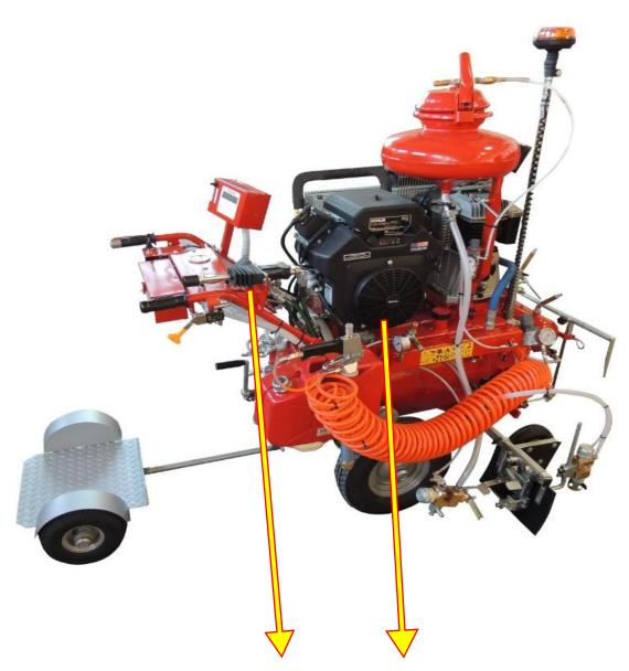
Increased 20.5 HP motor applied to self-propelled hydraulic drive by means of a variable displacement pump (P.P.V.)
